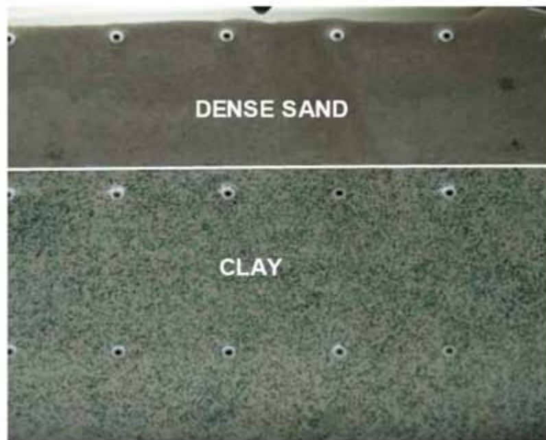
(a) Prior to spudcan installation
